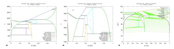
The magnification in the middle shows that with some GNUPLOT drivers one can use greek letters. In the right hand diagram we plot the entropy in the phases vs composition.
