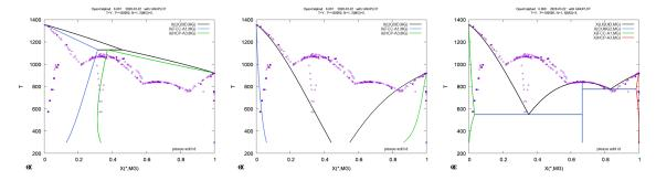
In the first diagram in the next set the Laves phase has been fitted and in the middle the solubilities in the FCC and HCP phases. The last diagram shows a metastable phase diagram without the intermediate phases, compare with the first two in the previous row! The example does not make a total fit to all data, that is left to the user.
