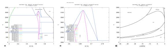
The middle diagram is a magnification of the congruent melting and the right hand plot has the oxygen potential as  $\log(p_{O_2})$  as the horizontal axis. The gaps are due to missing
